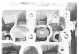
Using special tools, compress the valve springs and remove the two cotter halves ③ from valve stem.
