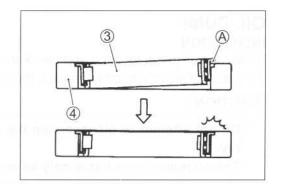
Install the guide ⑤ to the generator rotor with the arrow mark
