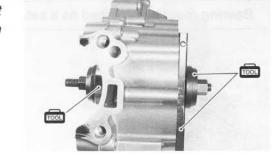
· Set the specified crankshaft journal bearings to the special tool.
