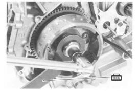
• Remove the generator rotor ② with the special tools.
