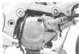
• Tighten all engine mounting clamp bolts to the specified torque. ( 3-14)
