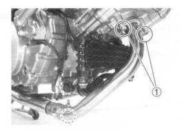
• Loosen the No.2 (Rear) cylinder exhaust pipe connector bolt.
