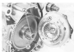
While holding the generator rotor with the special tool, tighten its bolt to the specified torque.
