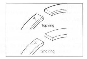
· Position the gaps of the three rings as shown. Before inserting each piston into the cylinder, check that the gaps are so located.
