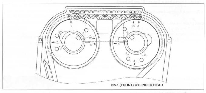
Install the dowel pins ①.
