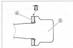
· Place the rear cylinder head on the cylinder.
