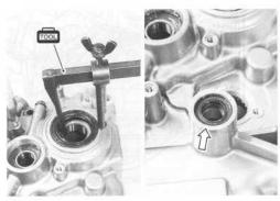
• Remove the bearing retainers ①.
