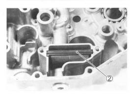
Clean the oil strainer with a compressed air.
