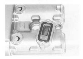
Apply THREAD LOCK to the bolts and then install the PAIR reed valve cover.
