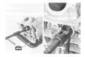
• Remove the valve spring retainer 4 and valve springs 5.
