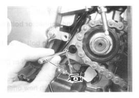
• Install the clutch cable to the generator cover temporarily.
