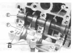
· Tighten the camshaft journal holder bolts to the specified torque.
