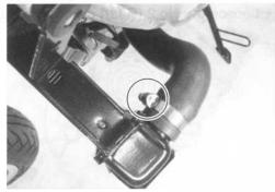
• Disconnect the horn coupler ① and cooling fan coupler ②.
