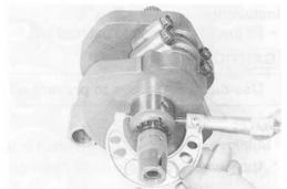
Select the specified bearings from the crankcase bore I.D. code. The crankcase bore I.D. code ① "A", "B" or "C", is stamped on the inside of each crankcase half.
