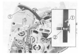
• Remove the rear cam chain ③ and cam chain drive sprocket
