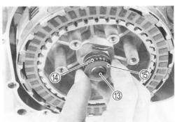
• Hold the generator rotor (crankshaft) with the special tool.
