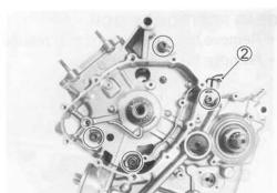
Separate the crankcase into 2 parts, right and left with the special tool.
