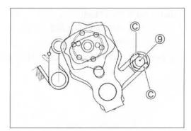
• Install the washer ① and snap ring ①.
