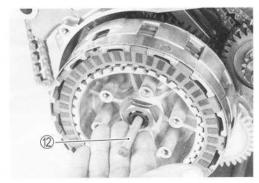
• Install the clutch push piece ③, the bearing ④ and thrust washer ⑤ to the countershaft.
