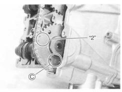
• The other arrow mark "2" on the exhaust camshaft sprocket should now be pointing straight up. Starting from the roller pin that is directly above the arrow mark "2" count out 16 roller pins (from the exhaust camshaft side going towards the intake camshaft side). Engage the 16 roller pin ① on the cam chain with the arrow mark "3" on the intake sprocket. ( 3-103)
