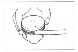
PATA Piston ring groove width
