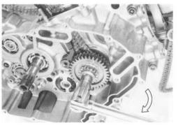
• Remove the water pump drive gear 1 and primary drive gear 2.
