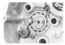
Install the gearshift cam stopper plate 6 with the gearshift cam pins A inserted into the gearshift cam stopper plate holes B.
