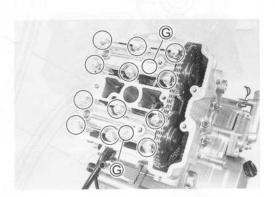
· Recheck the rear camshaft positions, intake and exhaust.
