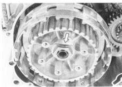
• Install the spring washer seat ⑦ and spring washer ⑧ onto the clutch sleeve hub correctly.
