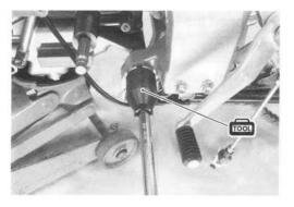
• Loosen the engine mounting thrust adjusters fully. NOTE:
