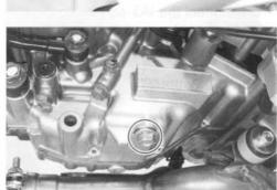
• Drain engine coolant. ( 2-20)
