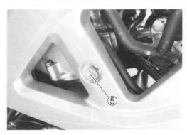
• Remove the engine mounting bolt 6.
