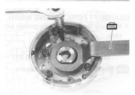
• Remove the one way clutch ① from the guide ②.
