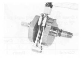
Remove the conrods, and mark them to identify the cylinder position.
