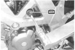
• Tighten all engine mounting bolts or nuts to the specified torque. ( 3-14)
