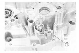
Check the operation of the oil pressure regulator by pushing on the piston with a proper bar. If the piston does not operate, replace the oil pressure regulator with a new one.
