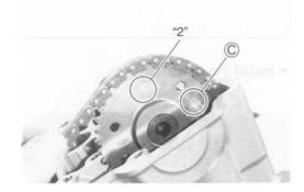
• The other arrow mark "2" on the intake camshaft sprocket should now be pointing straight up. Starting from the roller pin that is directly above the arrow mark "2" count out 16 roller pins (from the intake camshaft side going towards the exhaust camshaft side). Engage the 16th roller pin ① on the cam chain with the arrow mark "3" on the exhaust sprocket. (\$\sursymbol{L} \textsuperscript{3}-106)
