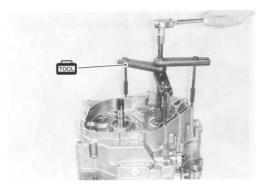
• Remove the O-rings 3 and dowel pins 4.
