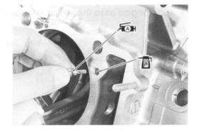
Install each of the oil jet (#14) to the left and right crankcase, as shown in the illustration.
