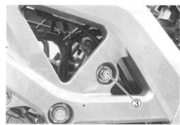
Remove the engine mounting thrust adjuster locknuts with the special tool.
