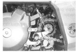
• Apply SUZUKI MOLY PASTE to the clutch release.
