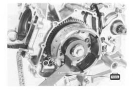
• Remove the primary drive gear bolt.
