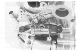
• Remove the rear exhaust pipe ® and gasket.
