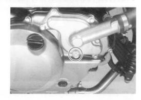
Loosen the throttle body clamp screws ① at the air cleaner box side.
