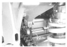
• Loosen the engine mounting clamp bolts ① and ②.
