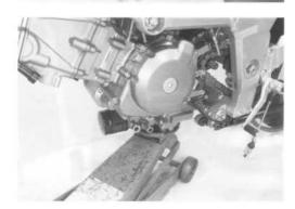
• Remove the engine mounting nuts 1 and 2.
