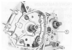
Remove the crankcase bolts and clamp ②.
