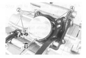
Apply engine oil to the sliding surface of the cylinders.
