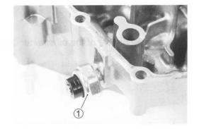
Apply SUZUKI BOND to the thread part of the oil pressure switch ① and tighten it to the specified torque.
